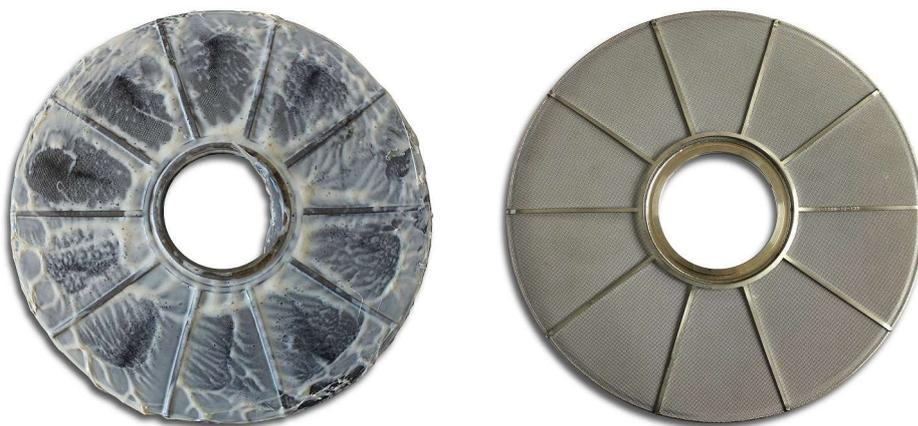
Filter disks before and after cleaning with vacuum pyrolysis, high-pressure water and ultrasound
