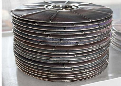
The thermal vacuum cleaning process first starts by melting off the adhering polymer from a filter stack in the assembled state. In a second step, the filter bundle is disassembled, broken down into individual discs and again subjected to vacuum pyrolysis. Precise post-treatment is carried out with high-pressure water and ultrasound
